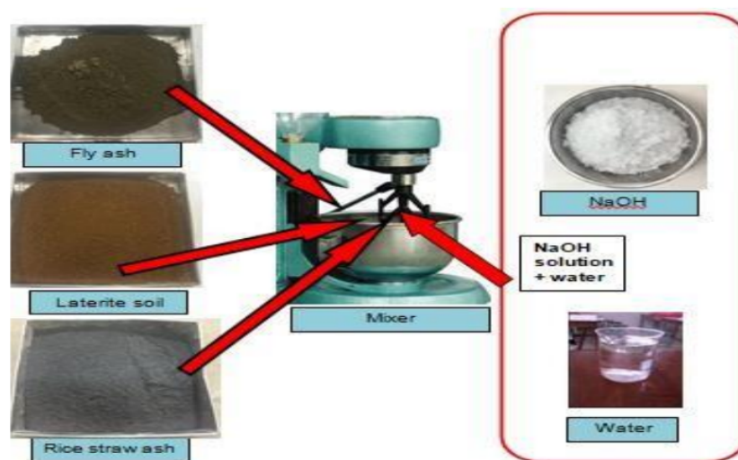
Figure 2. Mixing of geopolymer materials
