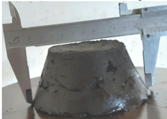
Figure 5. Flow of fresh geopolymer mortar
